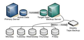
LifeKeeper Disk to Disk Backup with daily snapshots to disk and weekly backups to tape
